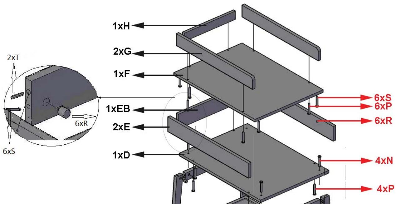
**Step 2 :** Use the frame of step 1, the top **D**, four bolts **N**, the back **EB**, both sides **E**, ten wood screws **P**, two wooden dowels (**T**), the cover **F**, six connectors **S**, six eccentrics **R**, the back **H** and both supports **G**
