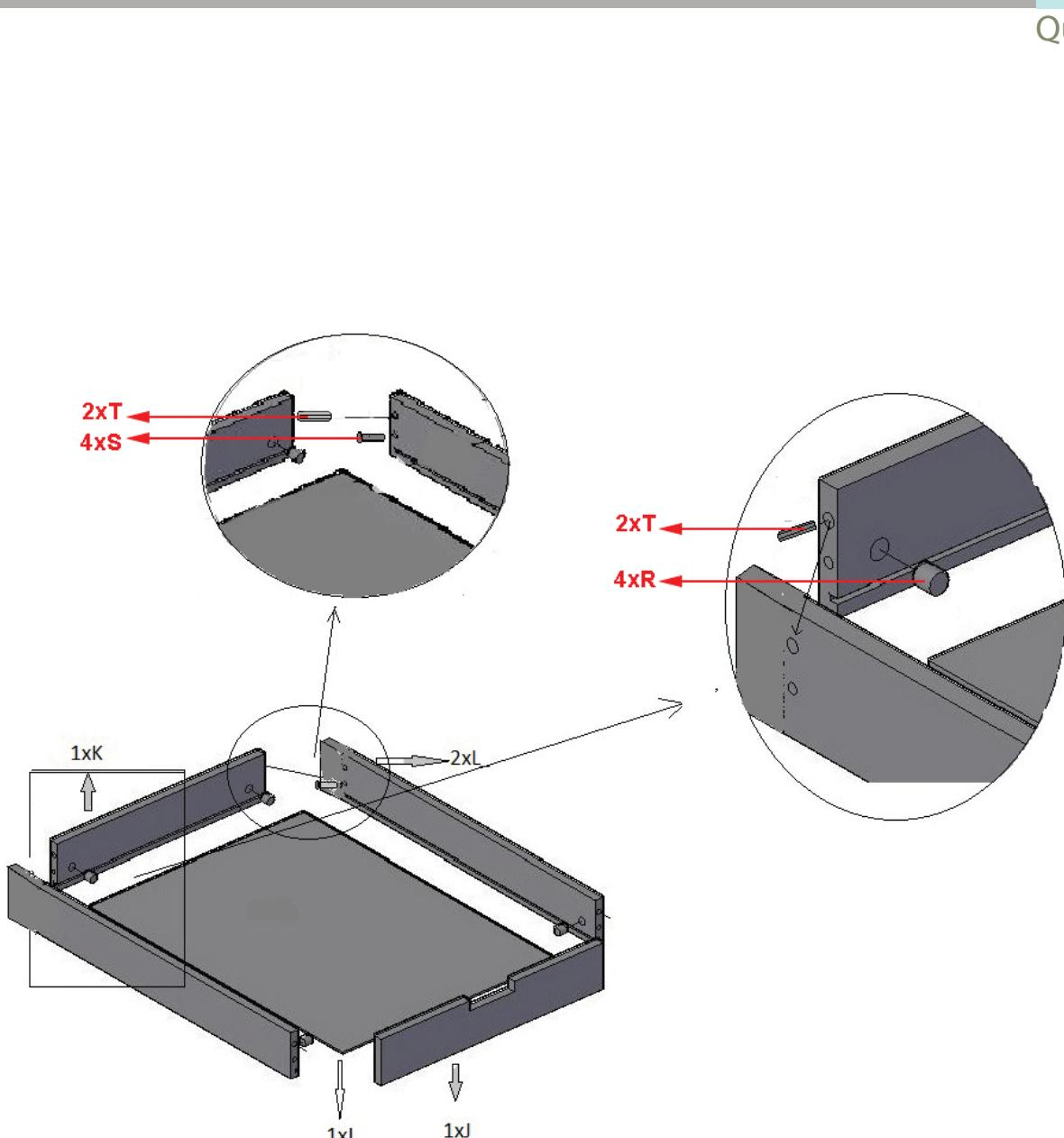
**Step 3 :** Use the mounted furniture, the drawer front **J**, the drawer back **K**, both drawer sides **L**, the drawer bottom **I**, four wooden dowels **T**, four connectors **S** and four eccentrics **R**
