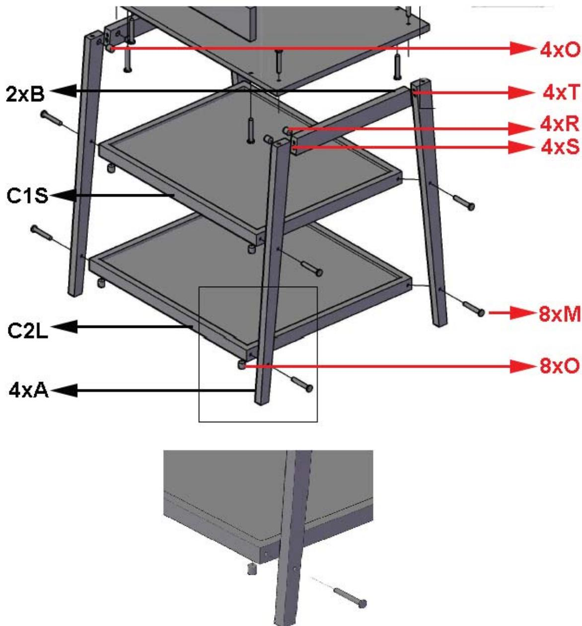
**Step 1 :** Use both crossbars **B**, four wooden dowels **T**, the four legs **A**, the shelves **C1S** and **C2L**, four eccentrics **R**, four connectors **S**, twelve cylindrical nuts **O** and eight bolts **M**
